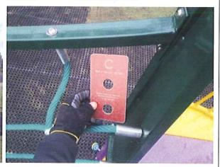
The item fails to meet the requirements for head and neck entrapment in between the net and handrail on the bridge BS EN 1176 Part 1
